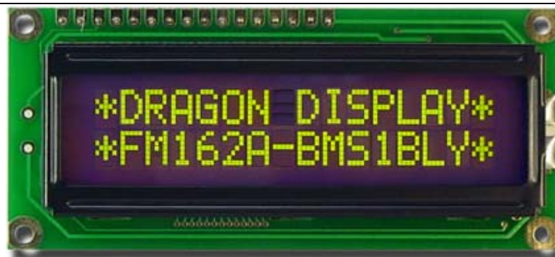
FM162A-BMS1BLY STN BLUE NEGATIVE TRANSMISSIVE YELLOW GREEN ARRAY LED BACKLIGHT
