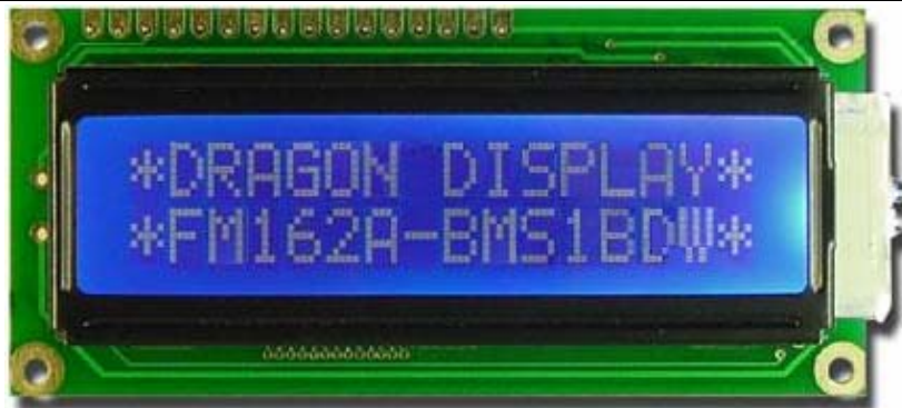
FM162A-BMS1BDW STN BLUE NEGATIVE TRANSMISSIVE WHITE EDGE LED BACKLIGHT
